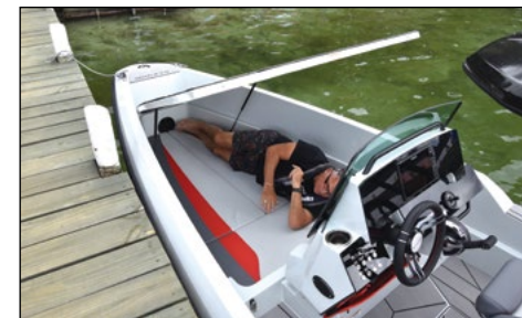
With a clip-on camper-style tent and the foredeck cushions, the area under the raised foredeck can be transformed into an occasional berth for overnighting.
